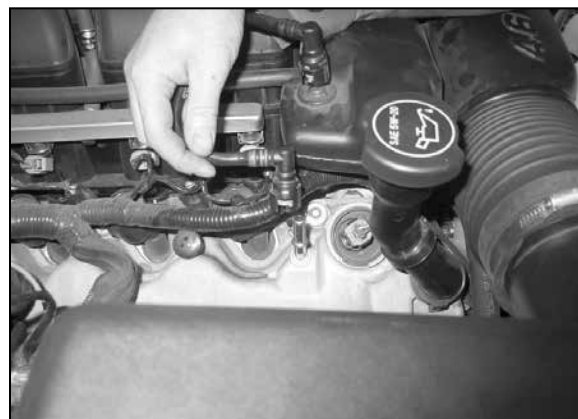
3. Rotate the green locking ring clockwise, then unhook the crank case vent hose from the valve cover.
