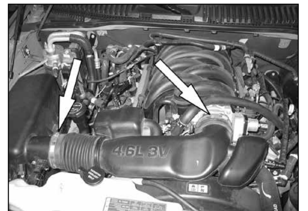
5. Loosen the hose clamps that secure stock intake tube to the throttle body and air box shown.
